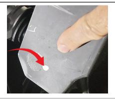
Route the hose through the hole, Leave about 1.5 to 2" of hose sticking out and cut off any extra.
