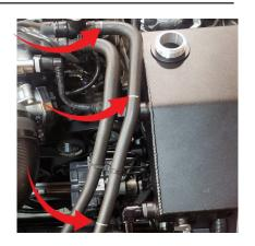
Remove or cut off the OEM zip tie hose tether that holds the 2 intercooler hoses together.
